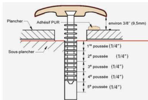
7. When finished applying adhesive, start again at the beginning of the moulding and push dowels 1/4" (6.4 mm) at a time until moulding is secure. Once moulding is in place, use a rubber mallet to tap on the top of each dowel. Use the pencil marks to reference where each dowel is located.
