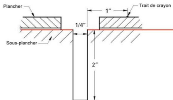
4. Carefully line up dowels with pre-drilled holes. Make adjustments to the dowel positions on the moulding if needed.
